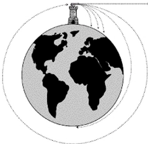
If a cannon ball were shot fast enough, it would go all the way around the Earth.
