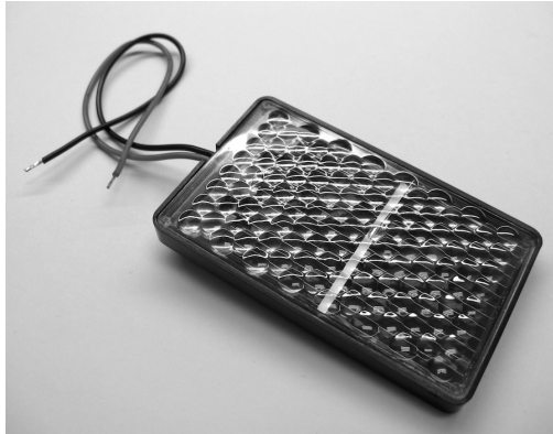
The type of solar cell used for the infrared detection circuit.
