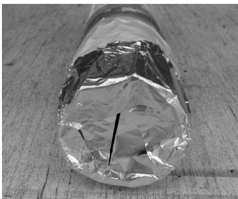
The slit end of a spectroscope. This end points at your light source.
