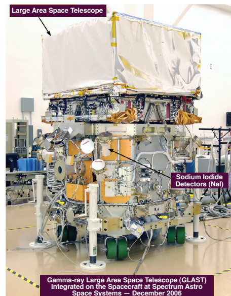
The LAT (silver box at the top) was integrated on the spacecraft at General Dynamics Advanced Information Systems in December 2006. Credit: NASA/General Dynamics Advanced Information Systems
