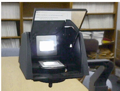
Close-up showing the placement of the diffraction grating on the overhead lens.
